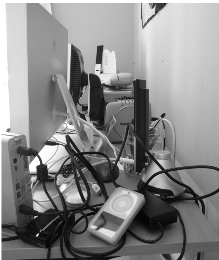
Figure 11. Interconnections allow selective upgrades at the expense of clutter
